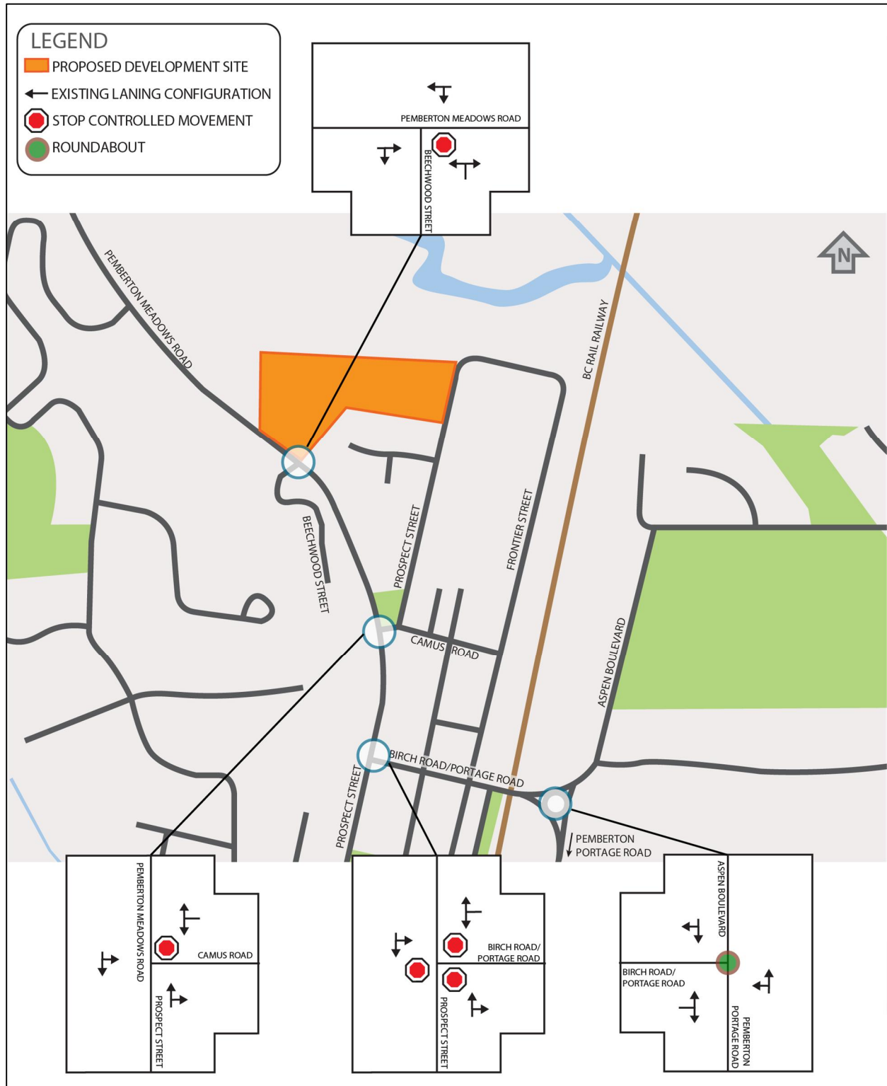
Figure 2-1: Existing Intersection Laning Configuration and Traffic Control
