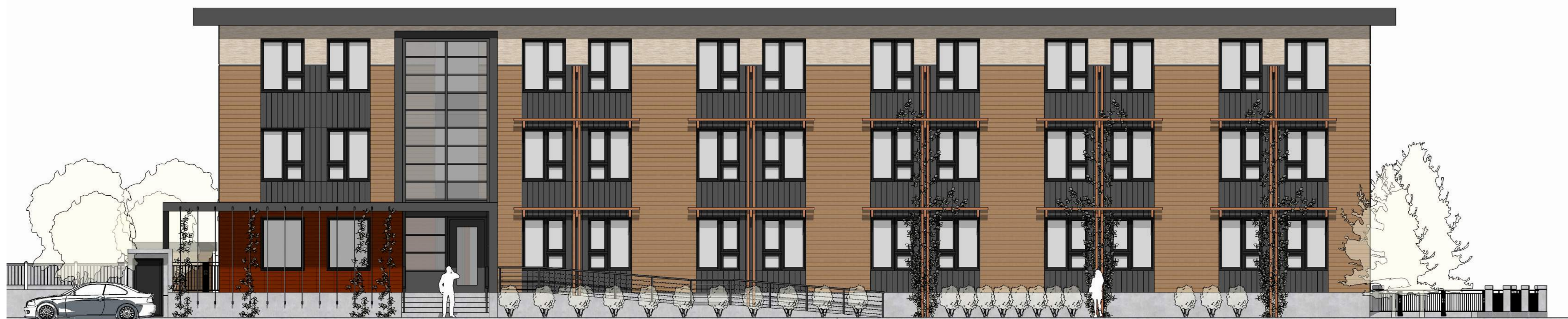
1 SOUTH ELEVATION SC: 1/4" = 1'-0"
