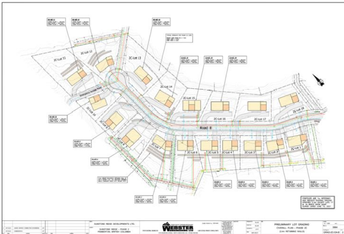
Figure 3: Phase 2C Plan for Retaining Structures
