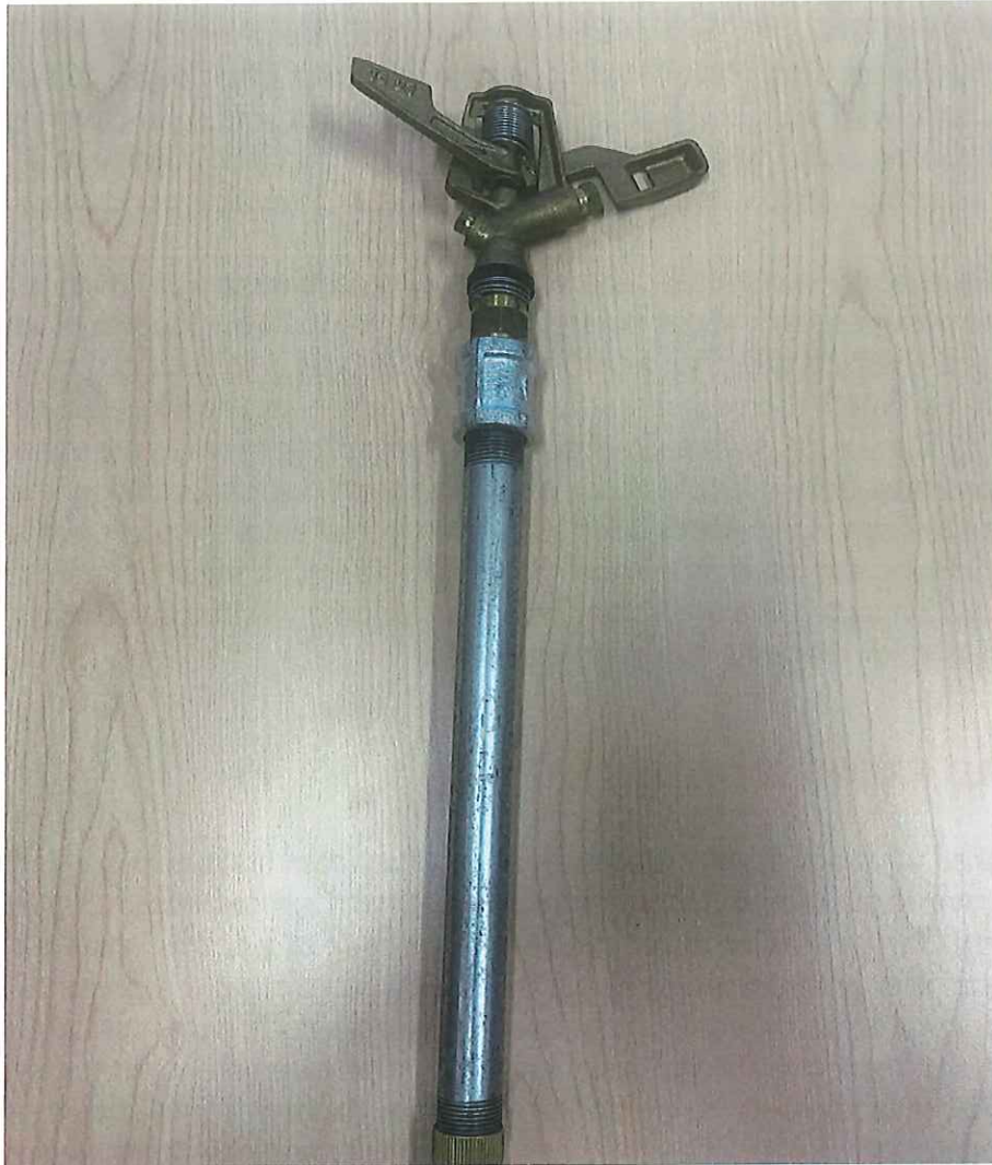
Figure 23: Rooftop sprinkler used in Logan Lake. (Source: District of Logan Lake)
