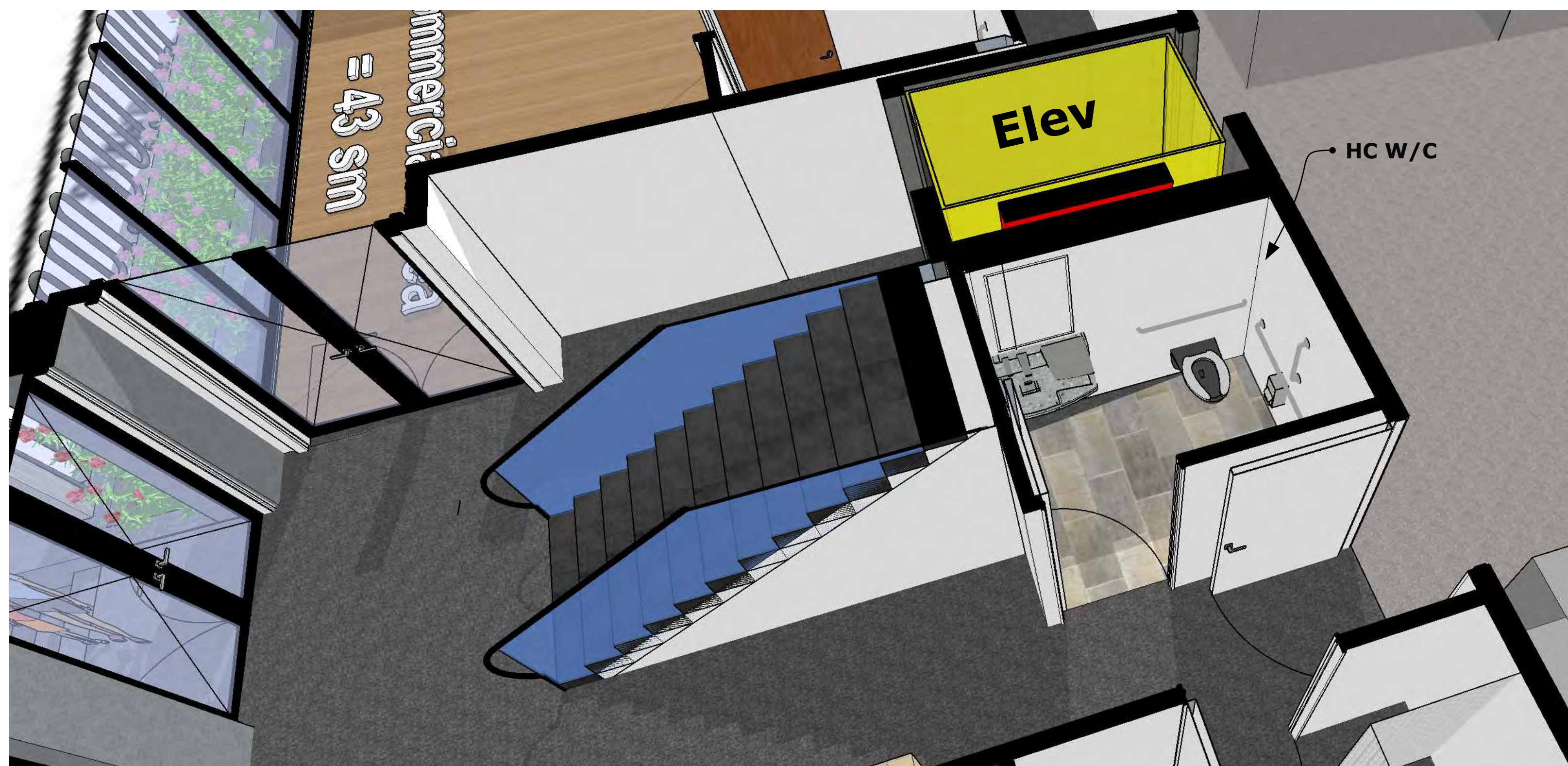
HC WC Under Main Stair
