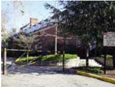
(Fig. 2.8) Manual gates cause inherent delays because personnel must dismount to unlock them or cut through chains. However, they can also help keep the fire access lane clear by preventing vehicle parking.
