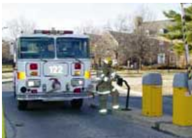
(Fig. 2.9) The delays caused by electronic gates can be minimized by providing the fire department with access cards or remove access controls.
