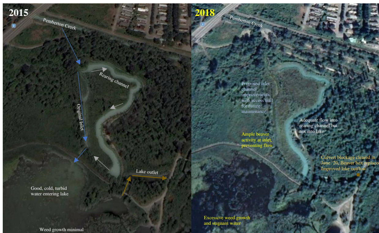
Figure 6 – One Mile Lake Inlet channel/ Fish Habitat Restoration Project
