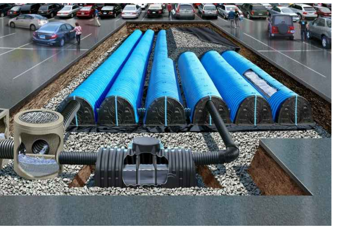
6 UNDERGROUND CISTERN Filtered stormwater will be collected in an underground cistern system for park irrigation.
