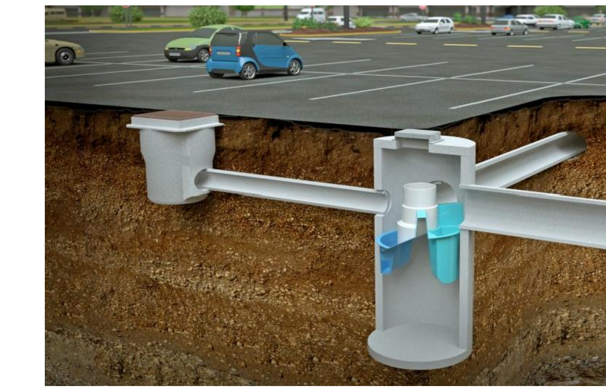
IMPROVED STORMWATER TREATMENT State of the art treatment utilities will be installed to efficiently purify overflows and stormwater runoff.
