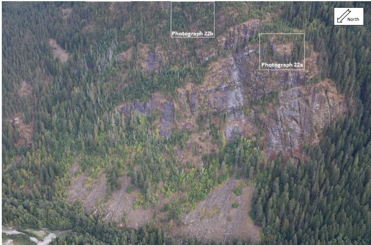
Photograph 24 DSGSD (Source ID 13) showing rock fall debris (weathered and covered with vegetation) at the base of a rock slope. Green River flows at the toe of the debris.
