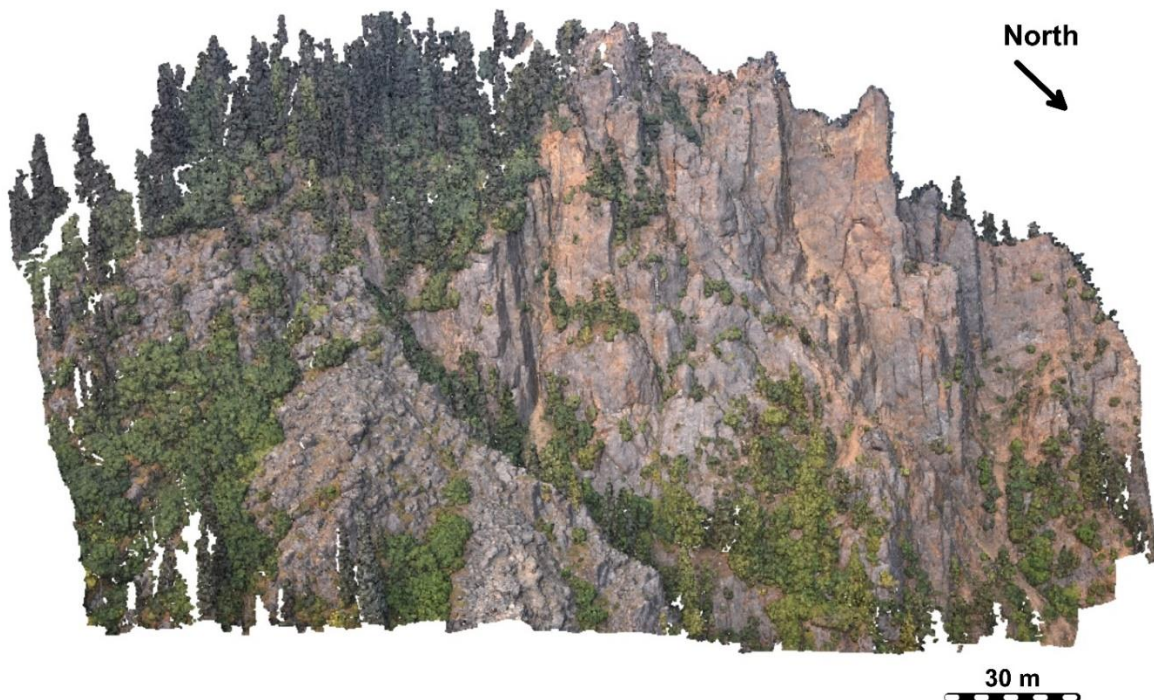
Figure B-1 3D model of a rock slope on the north face of Mount Currie
