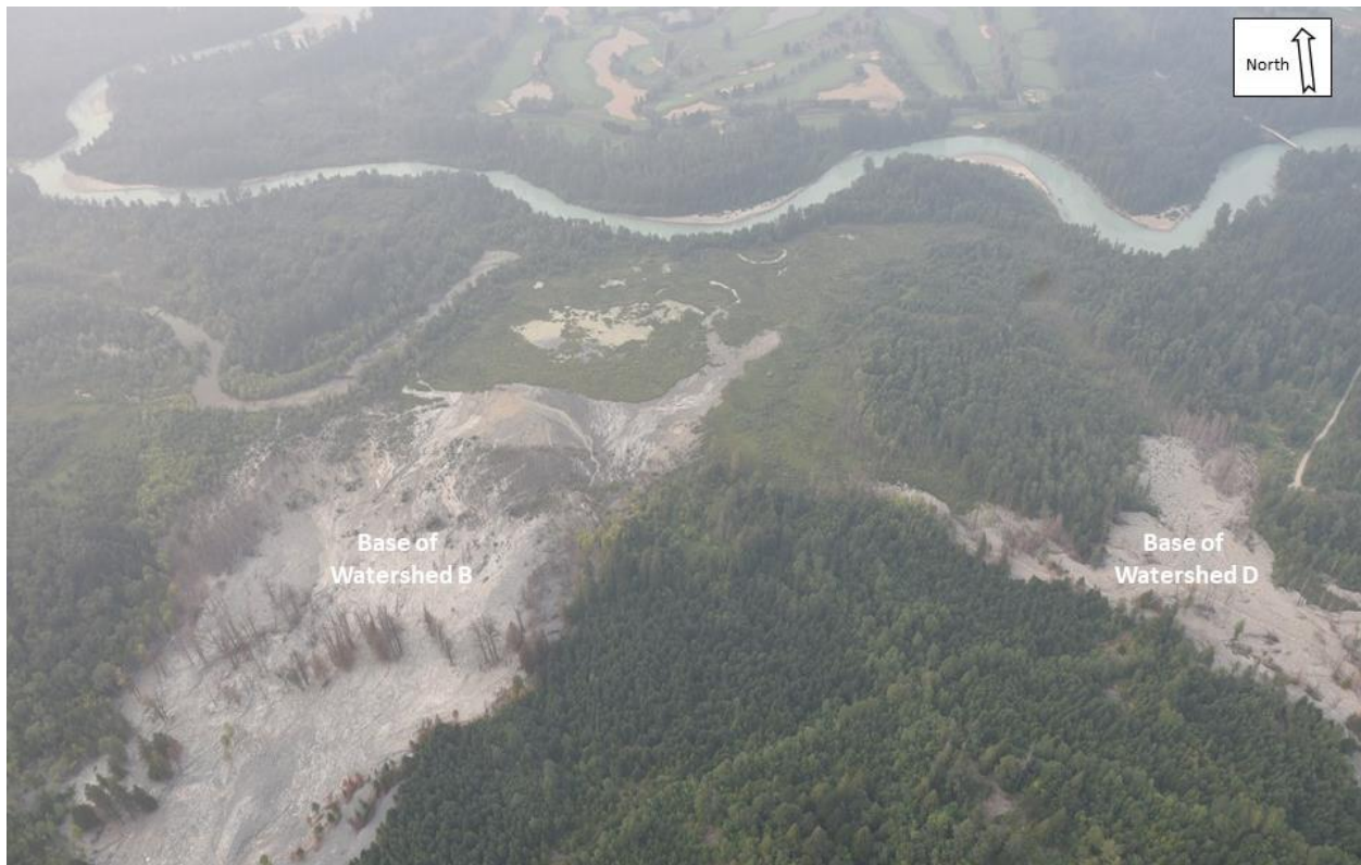
Photograph 45 View of the debris flow fans at the base of Watersheds B and D.
