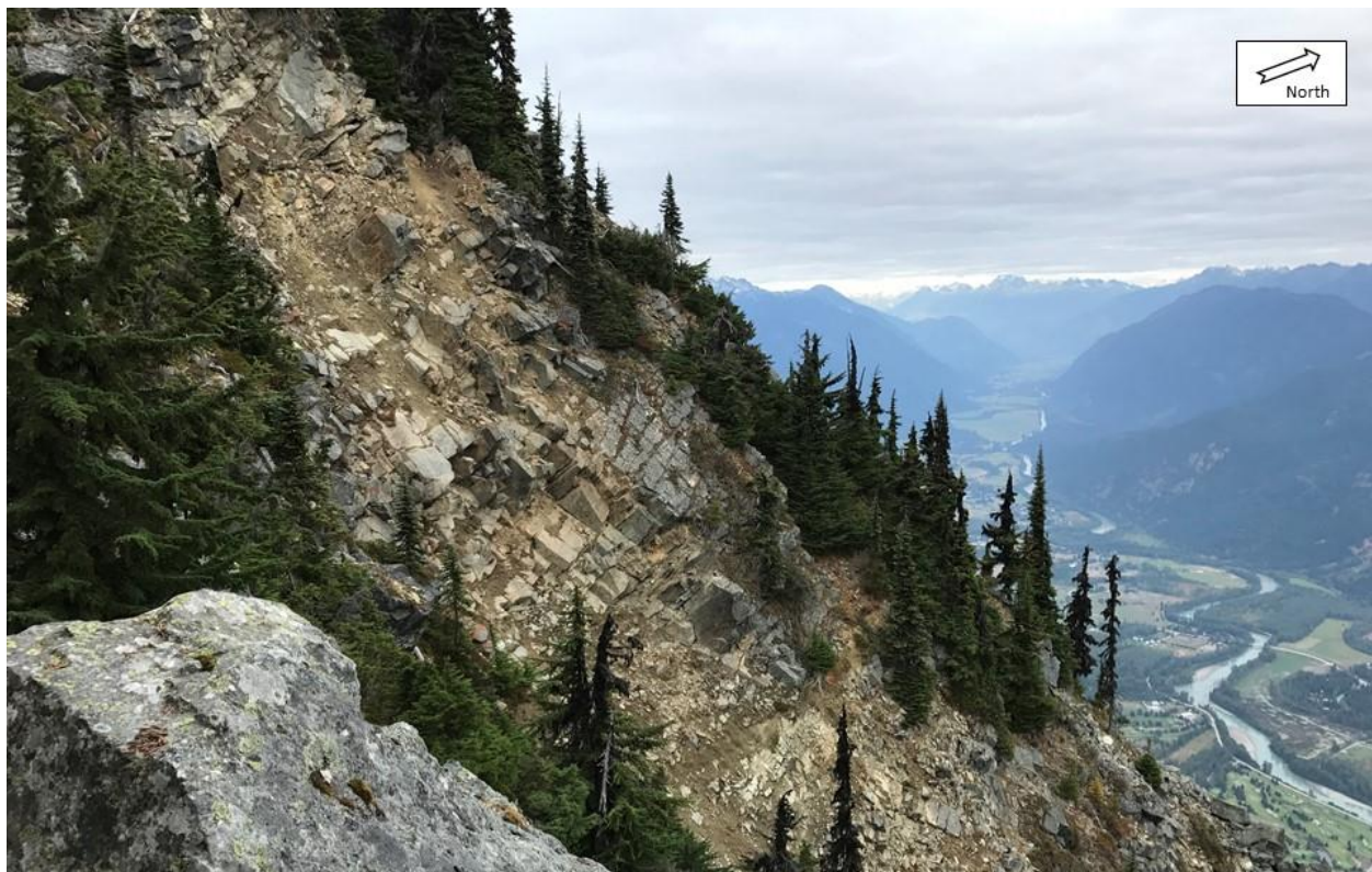
Photograph 15 Upper part of a section of Source ID 2b showing a disturbed rock mass and moderately dipping discontinuities.
