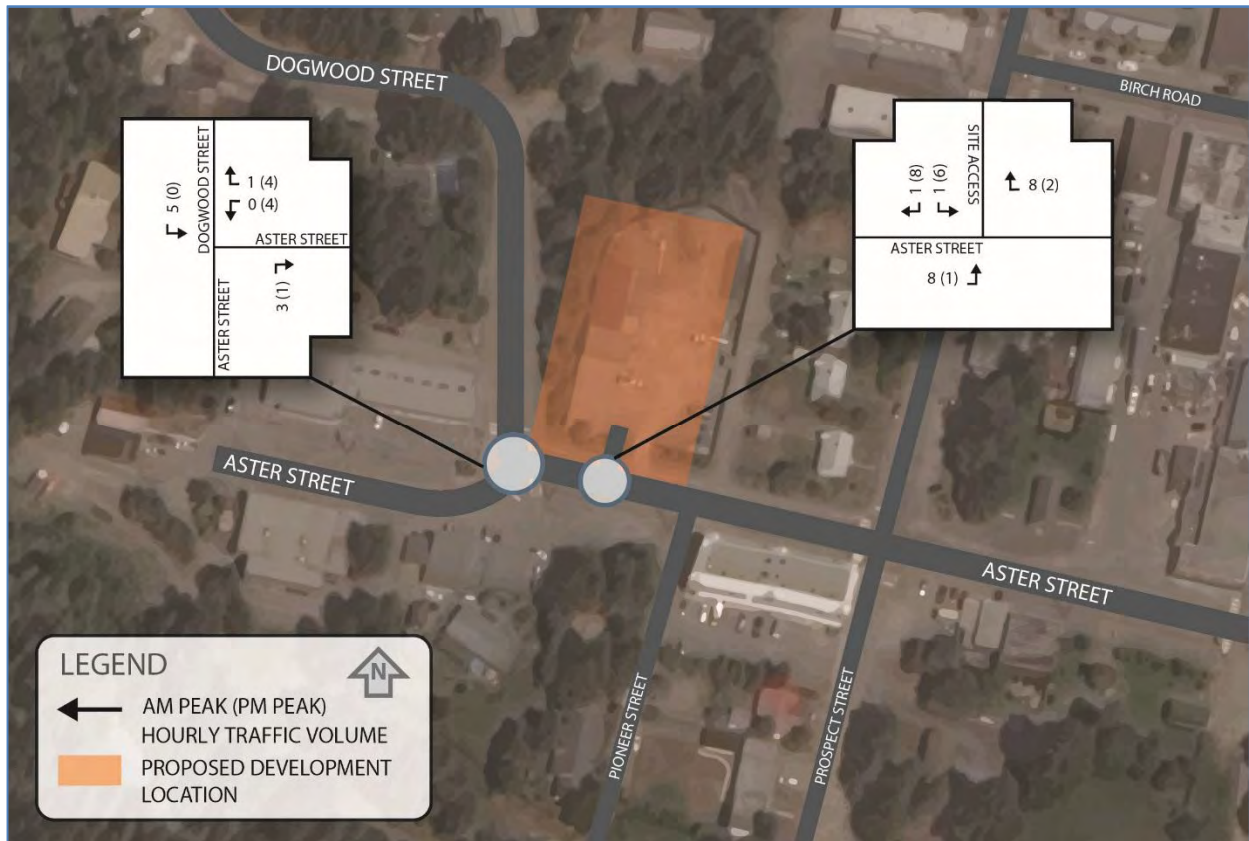
Figure 3-1: Forecast Site Generated Traffic Volumes
