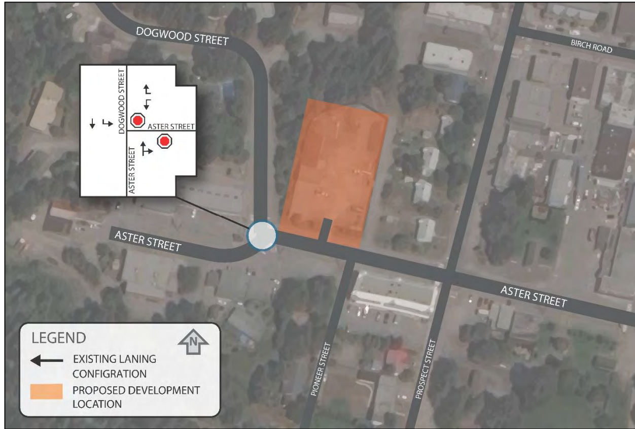
Figure 2-1: Existing Intersection Laning Configurations
